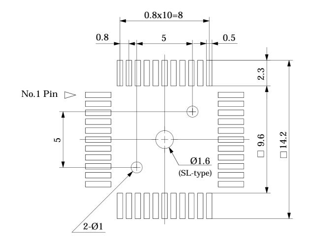
\* Recommended foot pattern shown on left is for NQPACK soldering. But please refer to IC package foot pattern recommended by IC manufacturer also, when the package is soldered on the same foot pattern.
