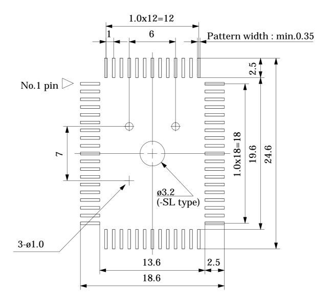
\* Recommended foot pattern shown on left is for NQPACK soldering.
