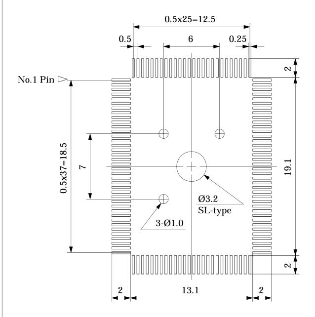
\* Recommended foot pattern shown on left is for NQPACK soldering. But please refer to IC package foot pattern recommended by IC manufacturer also, when the package is soldered on the same foot pattern.
