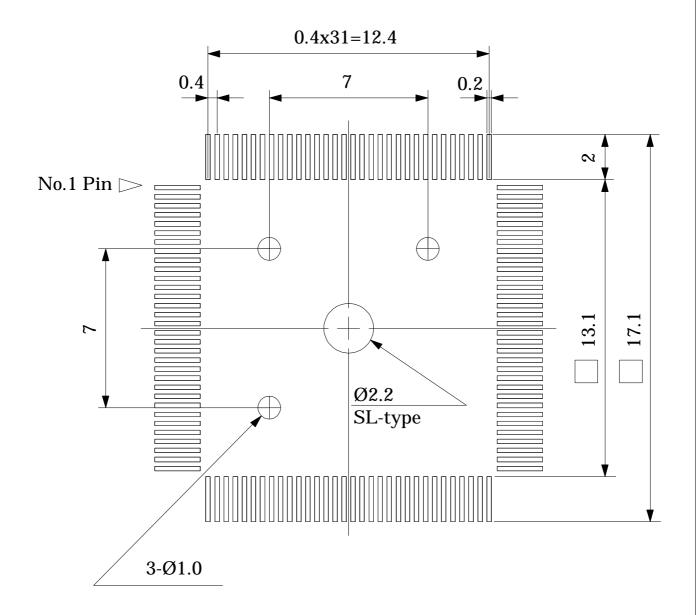
\* Recommended foot pattern shown on left is for NQPACK soldering. But please refer to IC package foot pattern recommended by IC manufacturer also, when the package is soldered on the same foot pattern.
