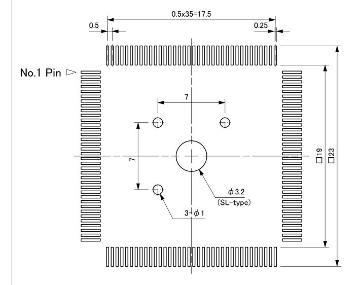
\* Recommended foot pattern shown on left is for NQPACK soldering.
