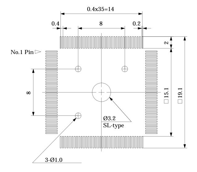
\* Recommended foot pattern shown on left is for NQPACK soldering. But please refer to IC package foot pattern recommended by IC manufacturer also, when the package is soldered on the same foot pattern.
